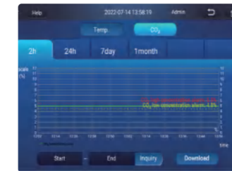
Real-time display of operation data & real-time display of temperature, for CO 2 concentration and O 2 concentration, and the data during the culture cycle can be viewed at any time.
